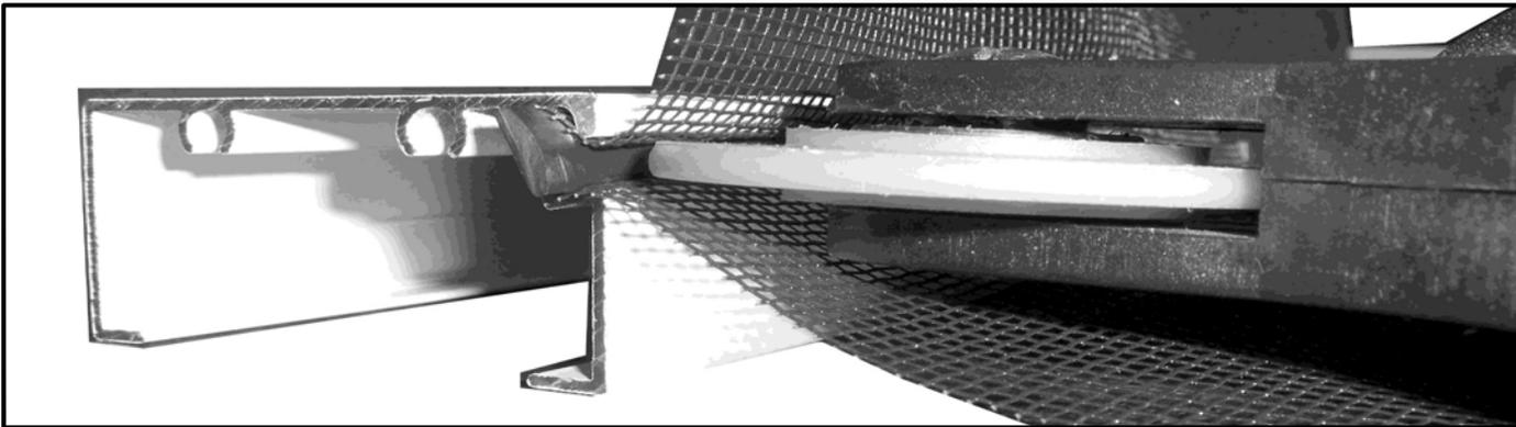
**NOTE:** "Flat edge" of spline seats in flat edge of channel.
