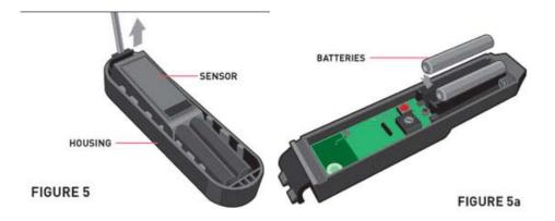
4. Remove the sensor from the housing using a small flat blade screwdriver. See figure 5
