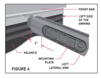
NOTE: The mounting plate when installed will face towards the Right Lateral Arm.
