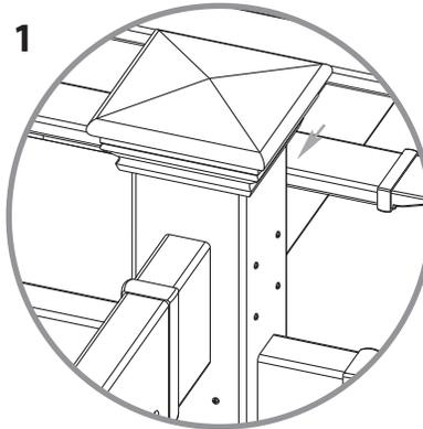
**First Shade Slat installed up against the vinyl column.**
