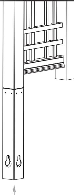
Slide the joiner of the 4x4 extension into the arbor posts.
