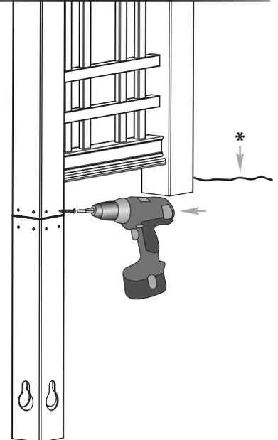
Screw all four sides of the arbor posts with 2 screws per side (repeat for all posts).
