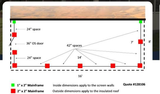
Walls are 8' tall with an 18" kickplate. Single outswing door quoted. Insulated roof is 3" thick
