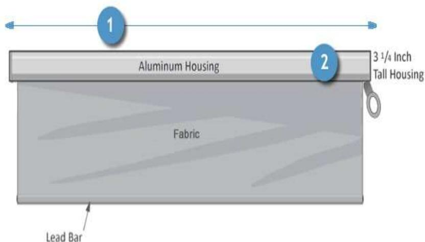
1. Measure for the width of your EasyShade. Manual EasyShades come in widths from 4 to 12 feet, in 1-foot increments. The total width is the width of the aluminum housing. (The fabric width is 4 inches less than the total housing width.)
