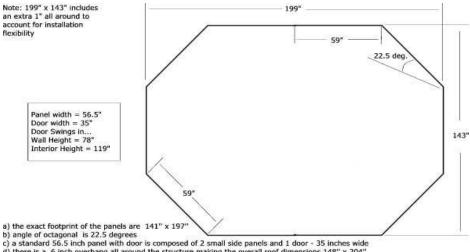
The drawing above shows some the measurements and details you may need to make sure you have the room necessary to install the Carousel on your deck or patio. The room SHOULD be screwed to a deck or patio for maximum strength in summer storms.
