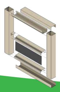
We provide you with extruded aluminum frames complete with screening and hardware that, when put together, create a permanent installation. The H122 mainframe has a .048" wall thickness and the H120 mainframe (for corners) has a .062" wall thickness.
