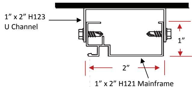
Install 1 "X 2" (H 121) at door head 80" from floor, or if your unit will have a chair rail and no kickplate, install 2" X 2" (H122) at door head 80" from floor. See illustration to the right.
