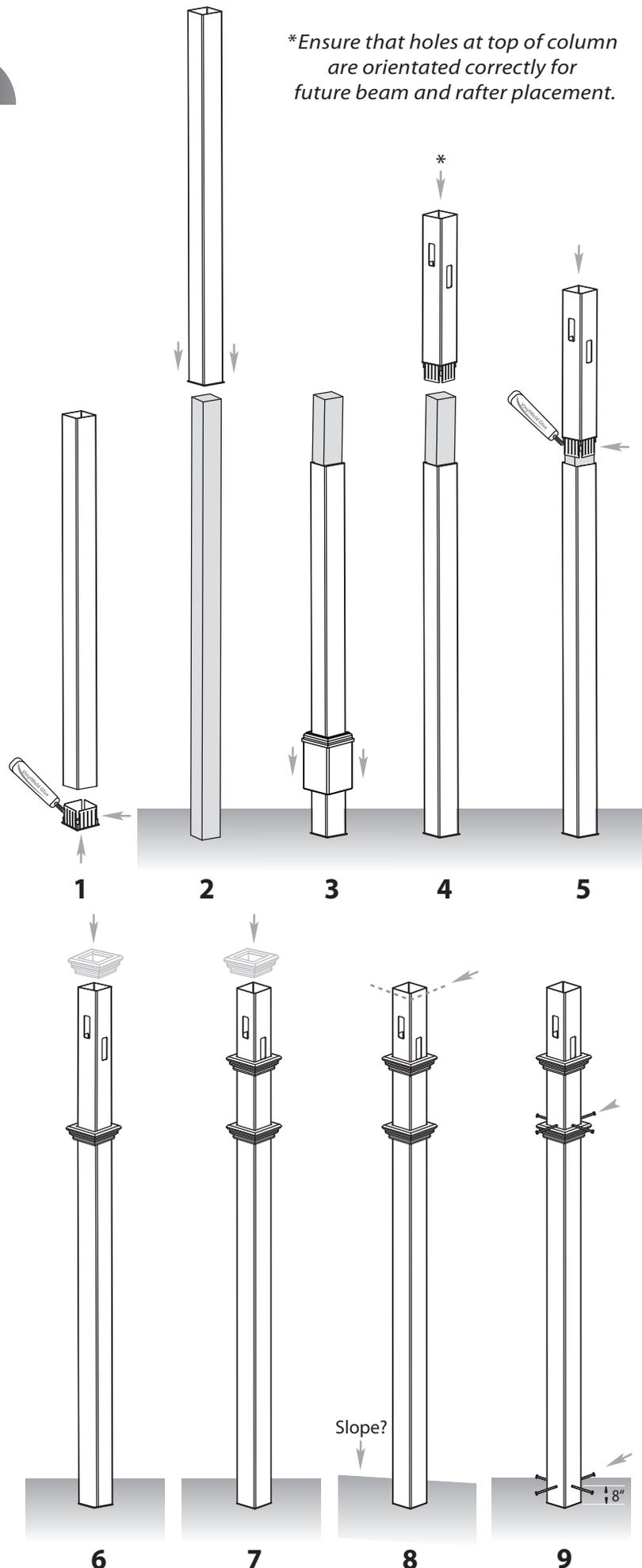
At this stage, the columns should be properly installed as per the following illustration, with the columns 110" apart.
