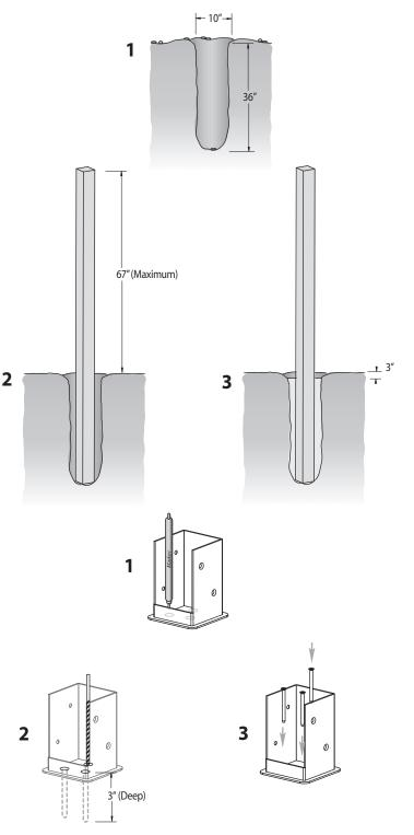
Wood Post Installation Using Bolt Down Bracket for
