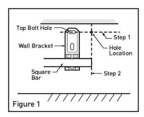
3. For Wood frame installation: At the intersection, drill a 1/8" pilot hole approximately 1-1/2" deep.
