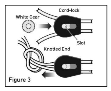
**7.** Slide the white round gear into the large (curved) open end of the cord-lock housing until the gear pops into place. Be sure that the part of the gear that protrudes is aligned with the slot in the cord-lock housing. Tie the two ends of the cord so that they cannot slide back through the cord-lock. Slide the cord-lock all the way towards the knot on the cord.
