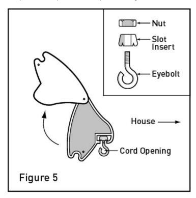
12. Slide the eyebolt assembly back against the side plate and tighten. Orient the eyebolt as shown in figure 5.
