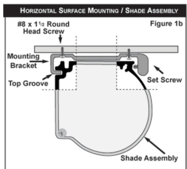
**STEP 1.** Determine the desired location for the mounting brackets, making sure that they are plumb and level. Using a pencil, mark the 2 hole locations in the bracket. Using a 1/8" bit, drill holes approximately 1-1/2" deep at both hole locations. Repeat for the mounting bracket on the other side, and the center mounting location on 10' models.
