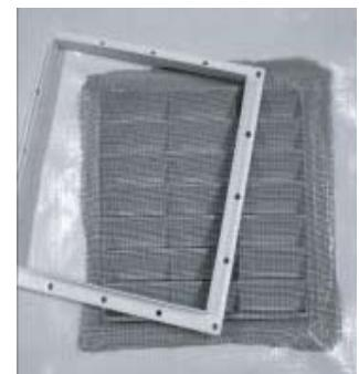
**Trim the excess screen and mesh from around the retainer.**
