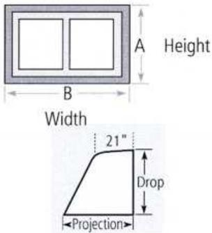
**Step-2:** Measure outside of window casing - edge to edge (B). If you mount the awning on the window casing (frame), this measurement is what you need. If you wish to mount the awning on the house wall then you need to add, at least, 1-1/2" on to each side to determine the final measurement. Awnings **cannot** be mounted on shutters.
